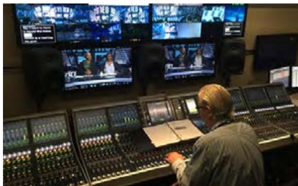
Atlas B unit's audio room houses a Lawo mc 2 66 MKII with 80 faders.
