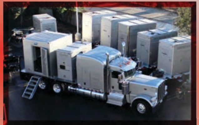
LB-15 with interchangeable POD UPS System and auto-start 168KW generator. The POD can be exchanged for a second 168KW to create a traditional TwinPack tractor.
