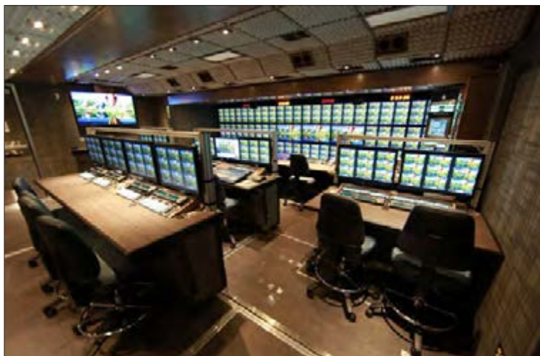
Game Creek Video's Encore mobile unit was among the first trucks to be built around an IP router, due to client Fox Sports' U.S. Open and Super Bowl needs.
