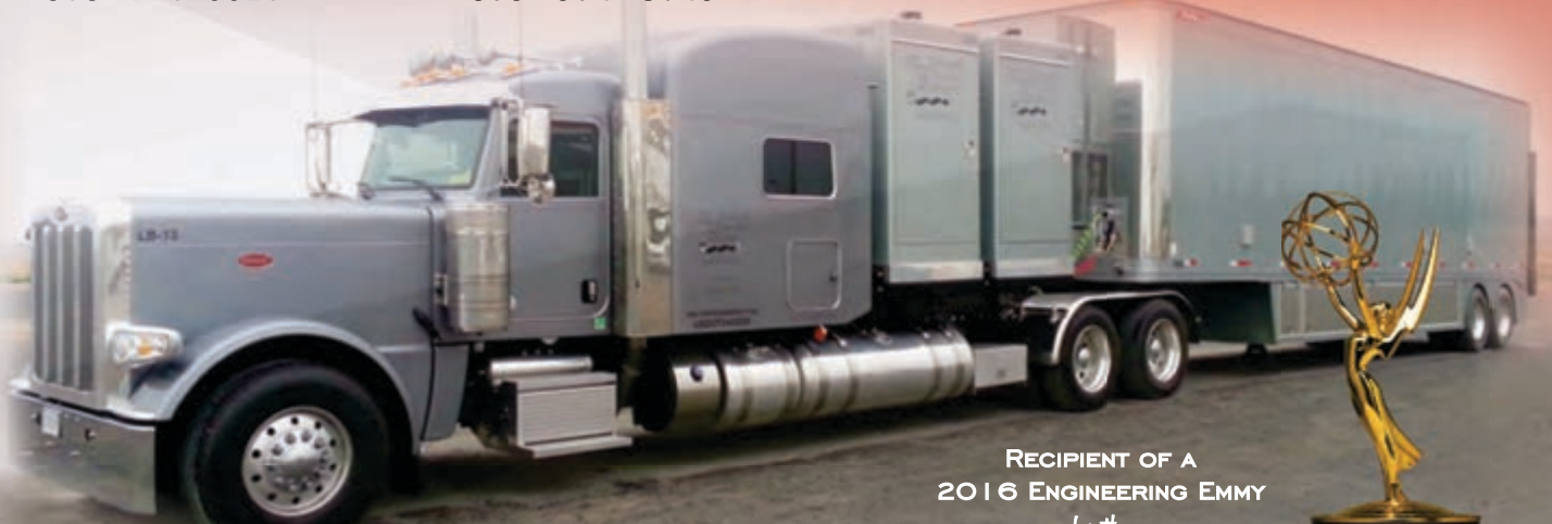
LB-13 with Twin 168KW movie quiet generators and Screens Trailer
