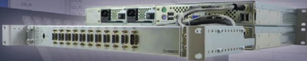
REAR MOUNTED AUTO CHANGE OVER REDUNDANCY IN 2 RACK UNITS
